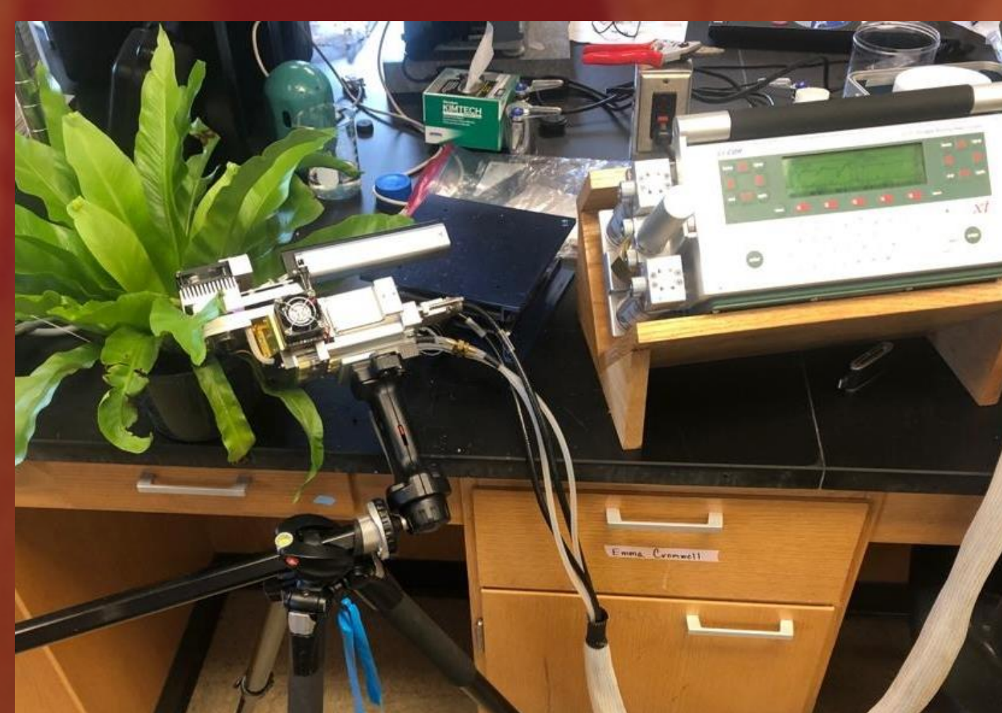
Fig. 2. LiCor photosynthesis gas analyzer measuring A. australasicum photosynthetic rate during drought experiment.
